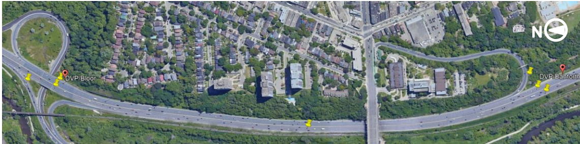
Figure 4-3 Location of chosen Bluetooth and VDS on DVP (Image source: Google Earth; red balloon represents Bluetooth detector, yellow pin represents VDS detectors)
