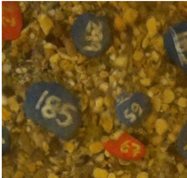
Figure 18: Planimetric view of bed material sediment and numbered immobile particles.
