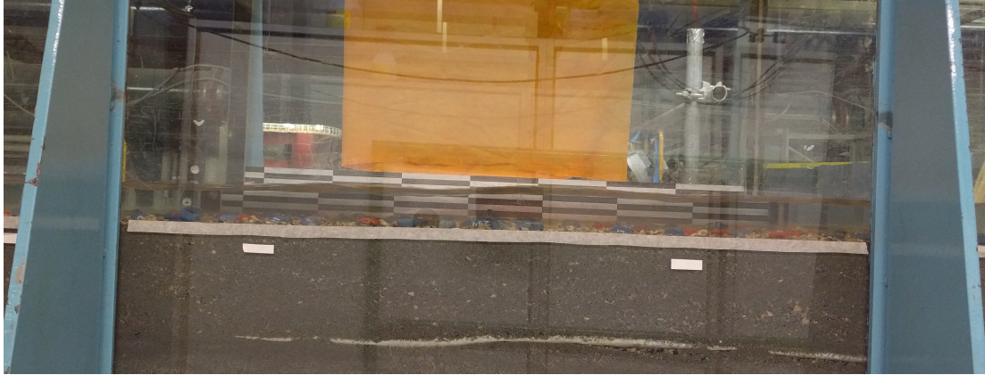
Figure 17: Side view of the flume in the middle of the study reach during a hydrograph. The grid behind the flume was defined at 1 cm and 10 cm vertical and horizontal spacings, respectively.
