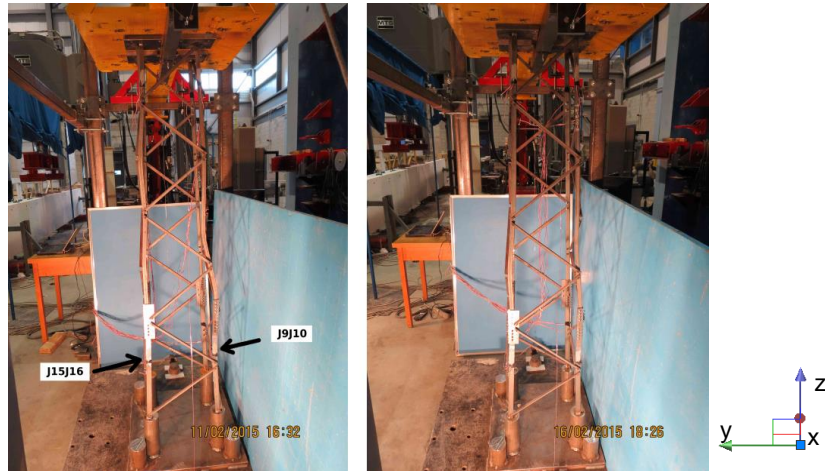
Figure 10: Experimental failure mode [Loignon and al. (2016)]
