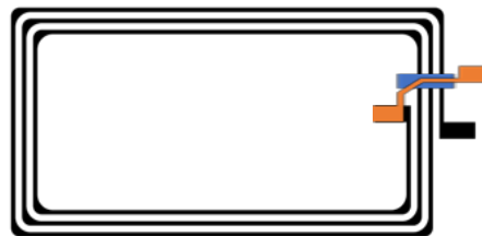
Figure 9 - RFID antenna 3-layer layout. In black is represented the first layer (antenna coil), in blue the insulant bridge (second layer) and in orange the last layer that pulls the inner pad to outside of the coil.
