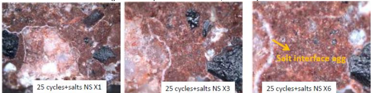
Fig. 9-8 – Samples CAC and CAC+, SEM after 25 cycles in direct contact with MS
