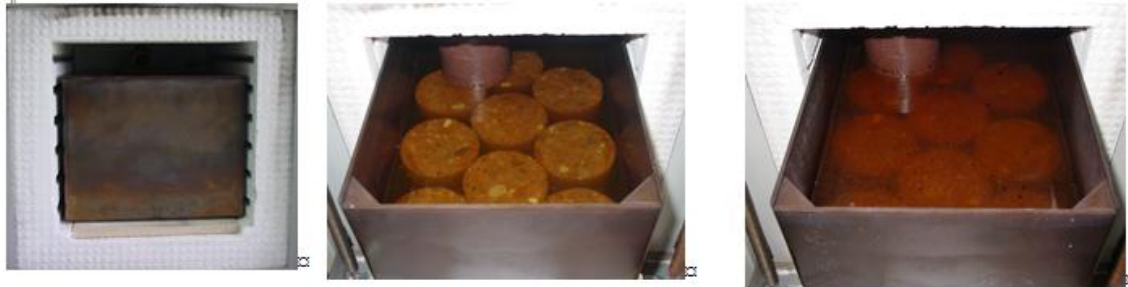
Fig. 9-3 – Samples CAC and CAC+ set in the oven in direct contact with molten salts
