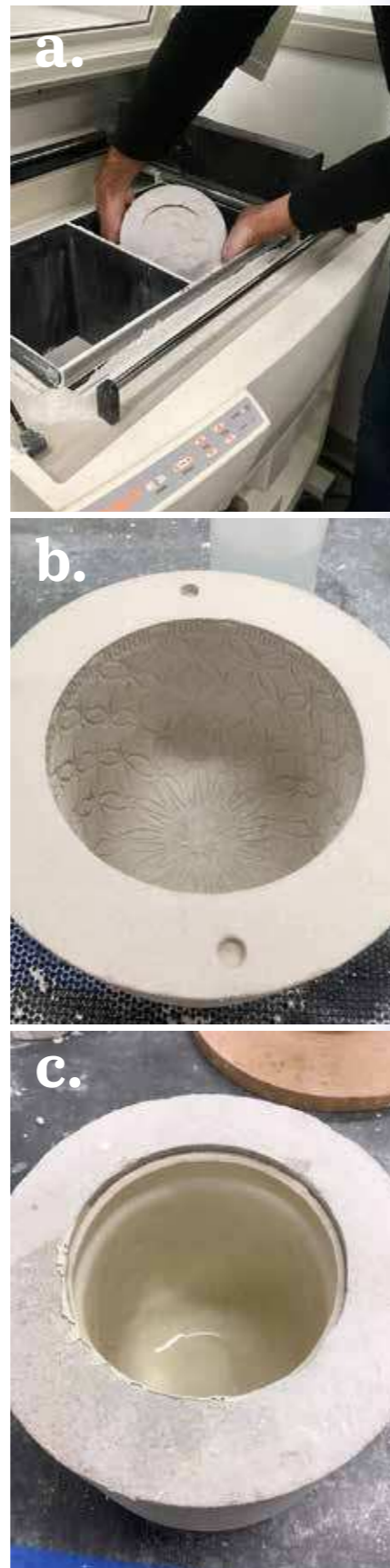
Figure 10. The process of making a two-piece 3D printed mould and using it for slip casting porcelain.
