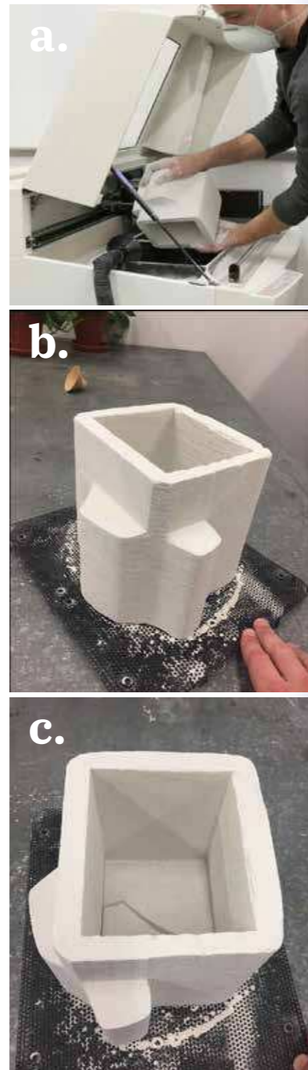
Figure 13. 3D printed moulds for glass casting, pre-firing.
