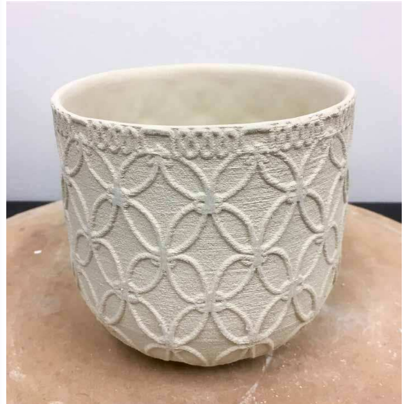
Figure 11. Cast porcelain cup from 3D printed mould.
