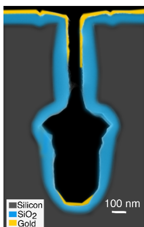
Figure 2.14 XSEM image of fabricated HED-TIE structure using spacer approach, prior to deposition of the organic channel.
