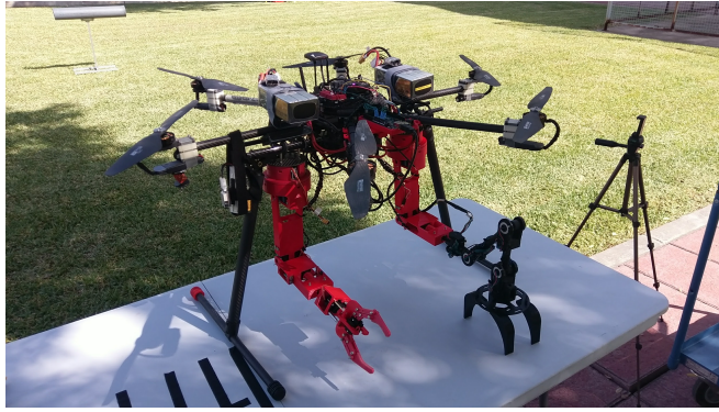
Figure 5.10 Dual arm aerial robot with gripper and docking tool..
