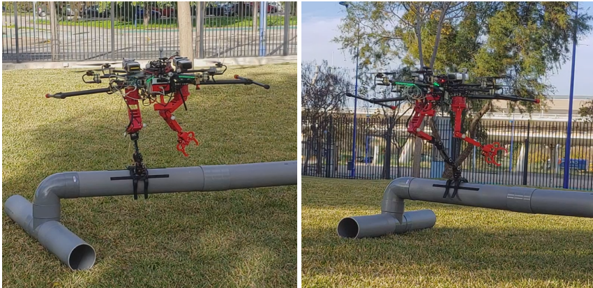
Figure 5.23 Outdoor experiments of the position based servoing of the manipulator using the position given by the docking tool.
