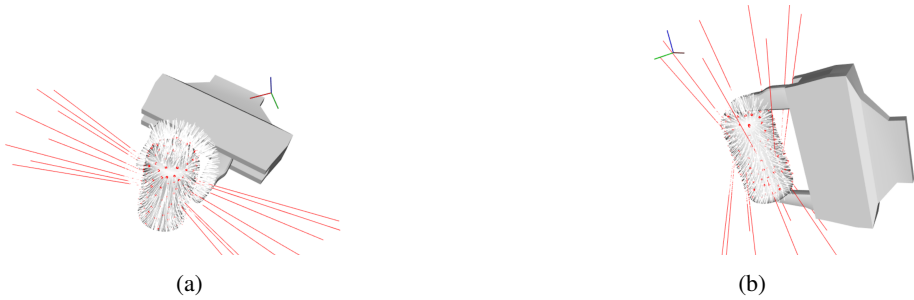
Figure 2.23 Examples of grasps generated on a cylinder. The reconstructed surface is represented by a gray mesh. Red lines belong to the convex cone of forces generated in the grasping points..
