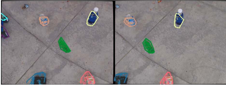
Figure 3.3 Left and right images with projection of the points belonging to candidate objects, surrounded by a convex hull. .
