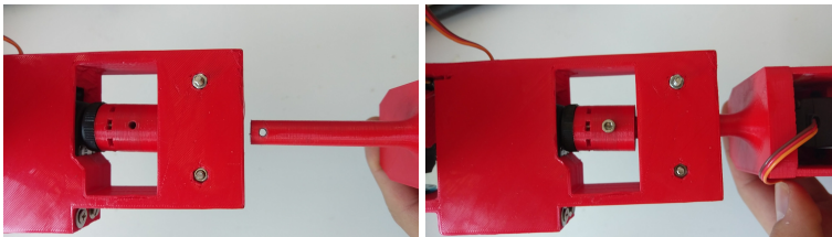
Figure 5.6 Quick release system for attaching different tools, i.e. the gripper or the docking tool..
