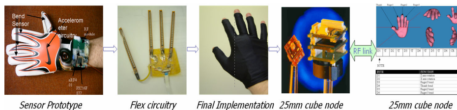
Fig. 5. 25mm Tyndall wireless sensor enabled glove prototype & GUI development cycle.
