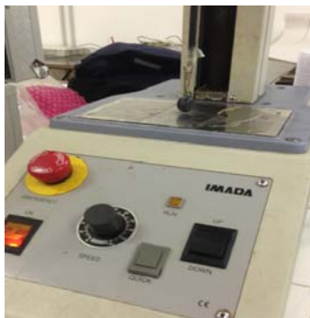
Figure 2 Dynamometer IMADA, DPS 5R for berry detachment force measurements
