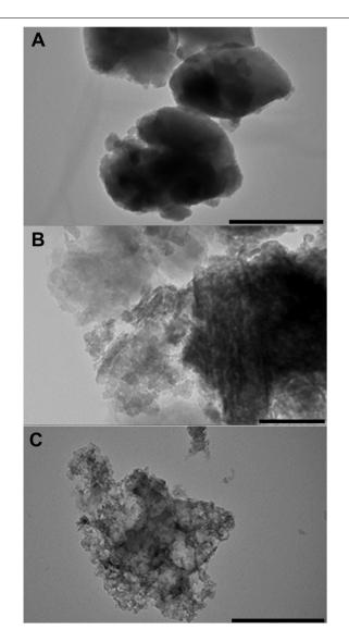
**FIGURE 1** | TEM images of three different zeolites (Chabazite –  $\bf A$ , Clinoptilolite –  $\bf B$ , and Natrolite –  $\bf C$ ) grinded in an electric mill up to particles of micrometer size. bar = 200  $\mu$ m.
