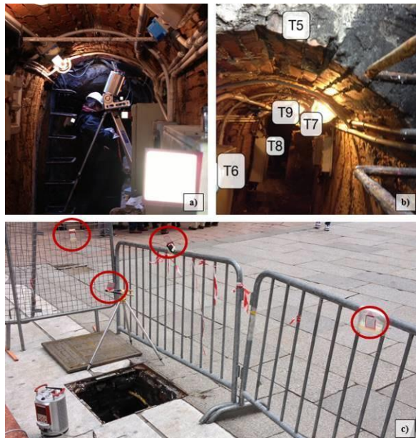
Figure 3. A phase of the underground surveying (a) and the placement of the targets used to align the clouds of the tunnels (b); some targets around the hatch used for the alignment of the above and the underground parts (c).
