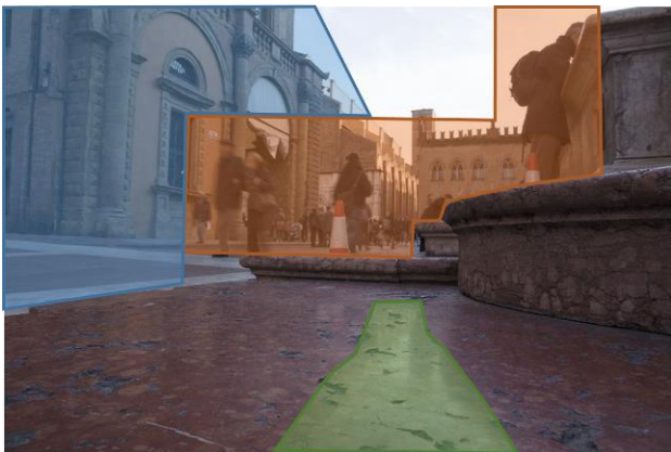
Figure 6. Image of the North-East corner of the fountain. Examples of problematic areas are highlighted: light reflections (green), changing of the background for people presence (orange) and out of focus objects (blue).
