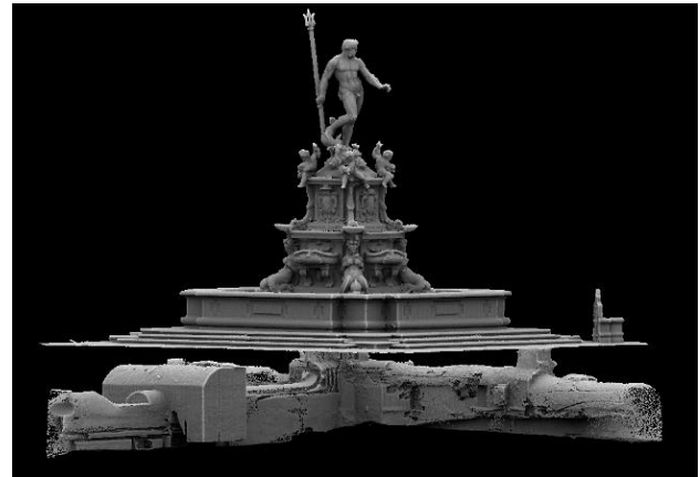
Figure 5. The 3D point cloud of the Fountain of the Neptune (above and underground in the same reference system), obtained by the TOF laser scanning.
