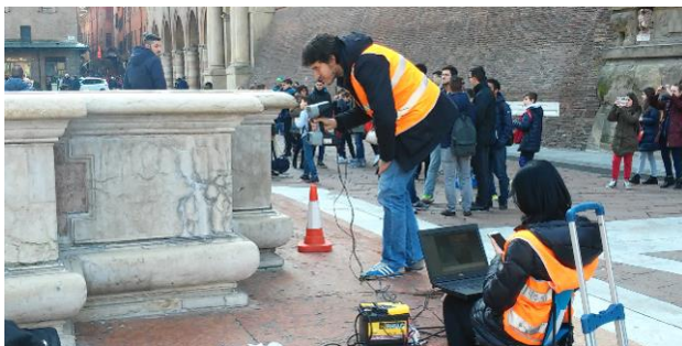
Figure 10. Surveying activities for the basement 3D modelling.
