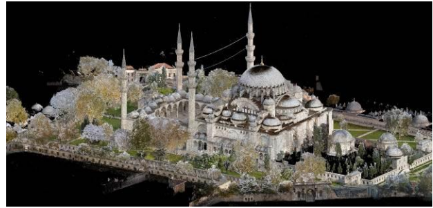
Figure 8. The view of colourized point cloud data in Riscan (Suleymaniye Mosque and complex exterior view)
