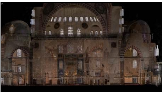
Figure 7. The view of colourized point cloud data in Riscan (interior view of Suleymaniye Mosque)
