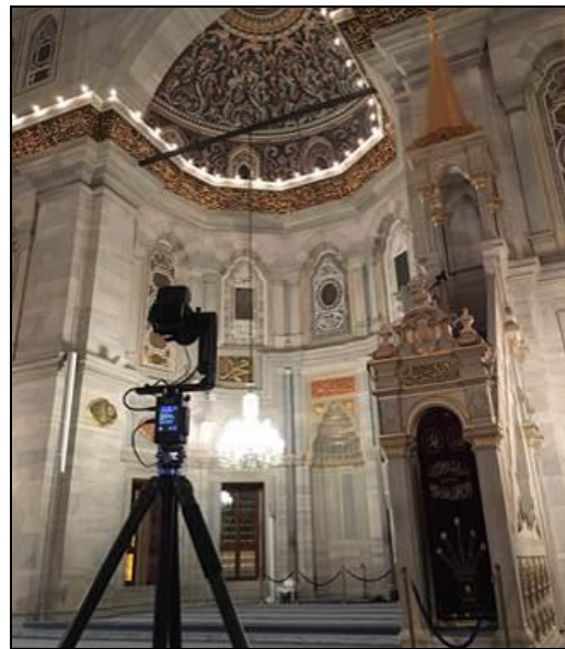
Figure 13. 360° panoramic image acquisition with Canon EOS 7D camera in the Suleymaniye Mosque
