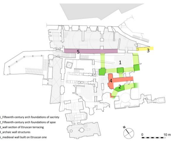
Figure 12. Basement plan; the new foundations of the transept in relation to the existing structures
