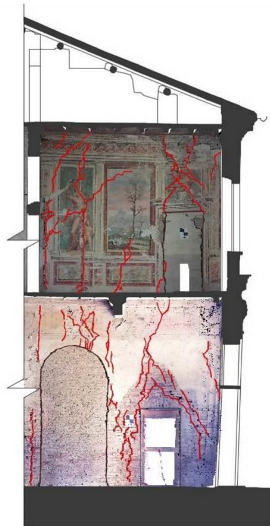
Figure 10: Details of the crack pattern.
