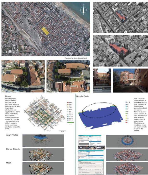
Figure 2. Comparative photogrammetric modelling phases: data acquisition from drone and Google Earth of G. Pascoli school.
