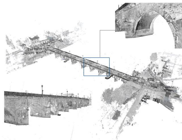
Figure 4. Azzone Visconti bridge's point clouds and its geometric irregularities.
