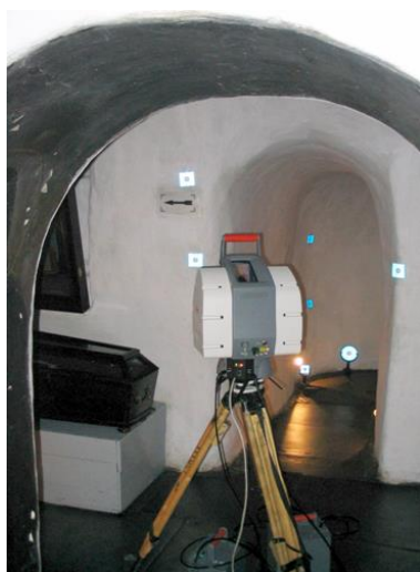
Fig. 6. Leica ScanStation and different orientation targets
