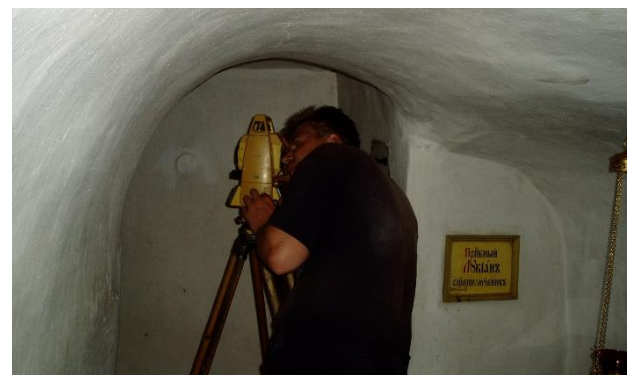
Fig. 3. Performance of geodetic measurements in caves
