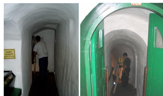
Fig. 4. Scanning stations georeferencing by free station method
