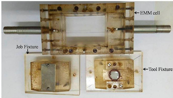
Fig. 2. Developed maskless EMM cell with tool and workpiece fixtures.
