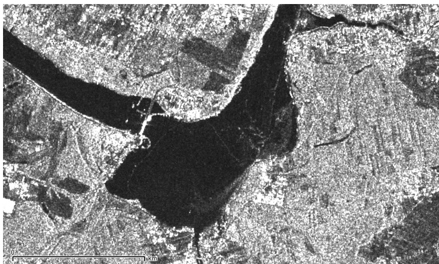
Fig. 8. Color composite from Sentinel-1 images recorded on January 9, 2017 shows continuous ice cover at Dębe reservoir with still visible embedded structure of pancake ice flow and lines of ice fractures
