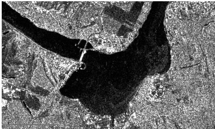
Fig. 6. Sentinel-1 image recorded on January 5, 2017 shows flow of pancake ice from Bug river to Dębe reservoir exposed to NW wind velocity 5 \text{ m} \cdot \text{s}^{-1}
