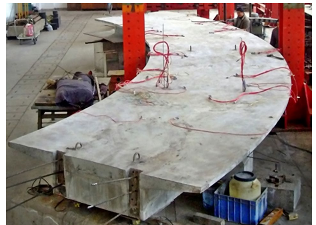
Figure 1. The large-curvature PCCBG bridge mode
