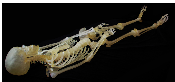
Figure 10. A plastic copy of the three-dimensional mummy reconstruction made by the laser stereolithography
