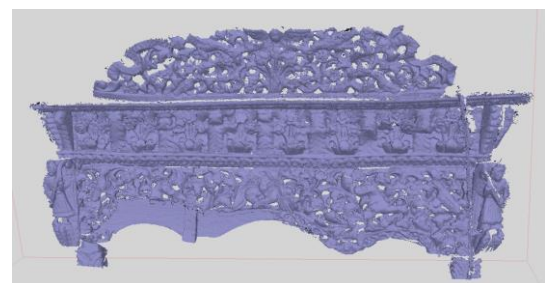
Fig. 4a Polygonal surface derived from the SfM procedure
