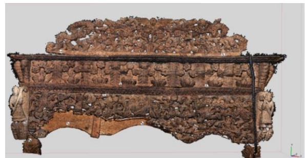
Fig. 3b Correct point cloud produced using SfM procedure with manually measured tie points (about 4.000.000 points)
