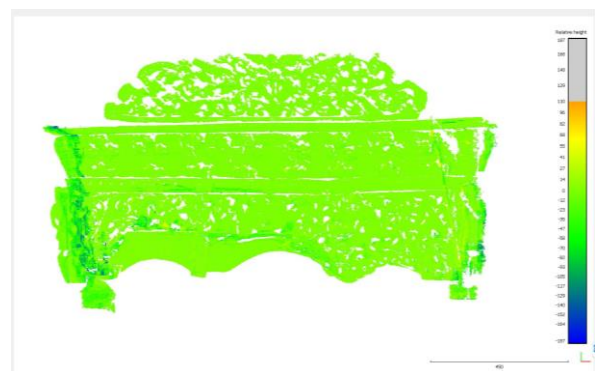
Fig. 6c Mesh-to-mesh volume comparison between the SfM and laser derived surfaces
