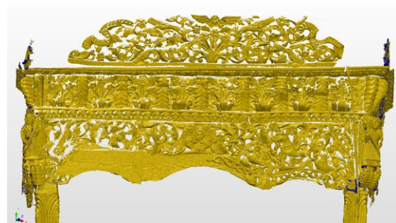
Fig. 4b Polygonal surface derived from the scanning procedure
