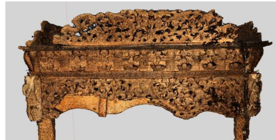
Fig. 3a Point cloud from automatic SfM procedure without manually introduced tie points
