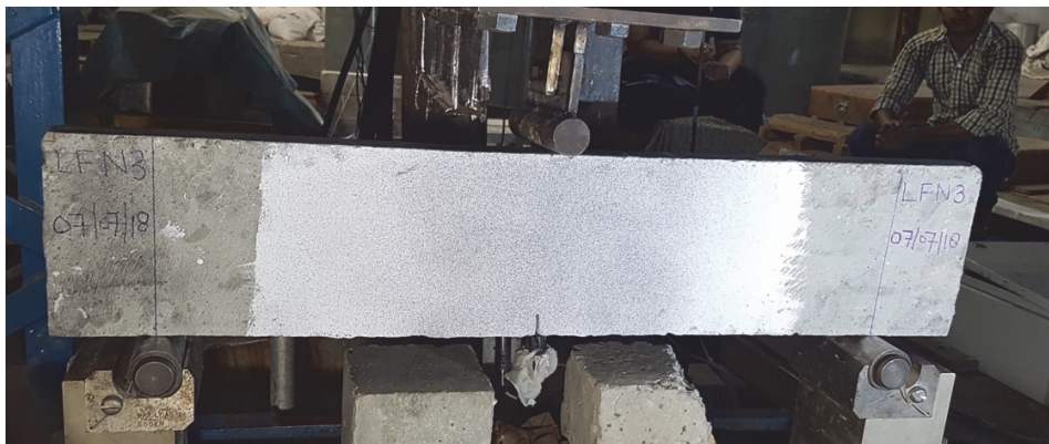
Figure 3: Fatigue test set up for three-point bending
