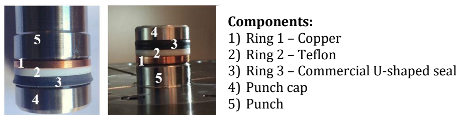
Figure 3: Bridgman seal on (a) upper and (b) lower punches.
