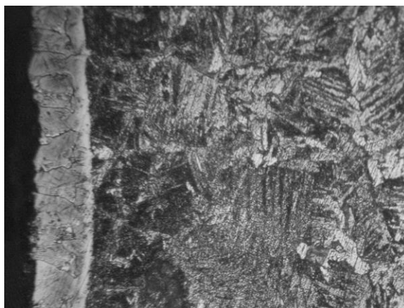
Figure 2 - Carbide layer after steel 20 saturation by molybdenum, x200
