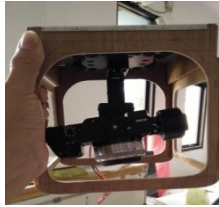
4(a) : Casing, Gimbal and camera
