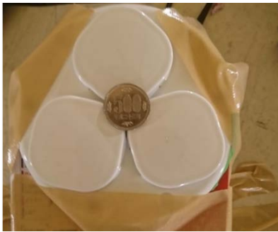
Fig. 5. Three-element array antenna
