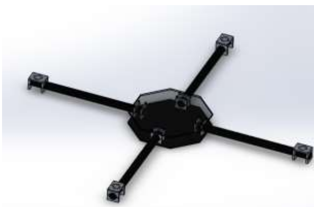
Fig. 11. Preliminary design of the frame built in carbon fiber.
