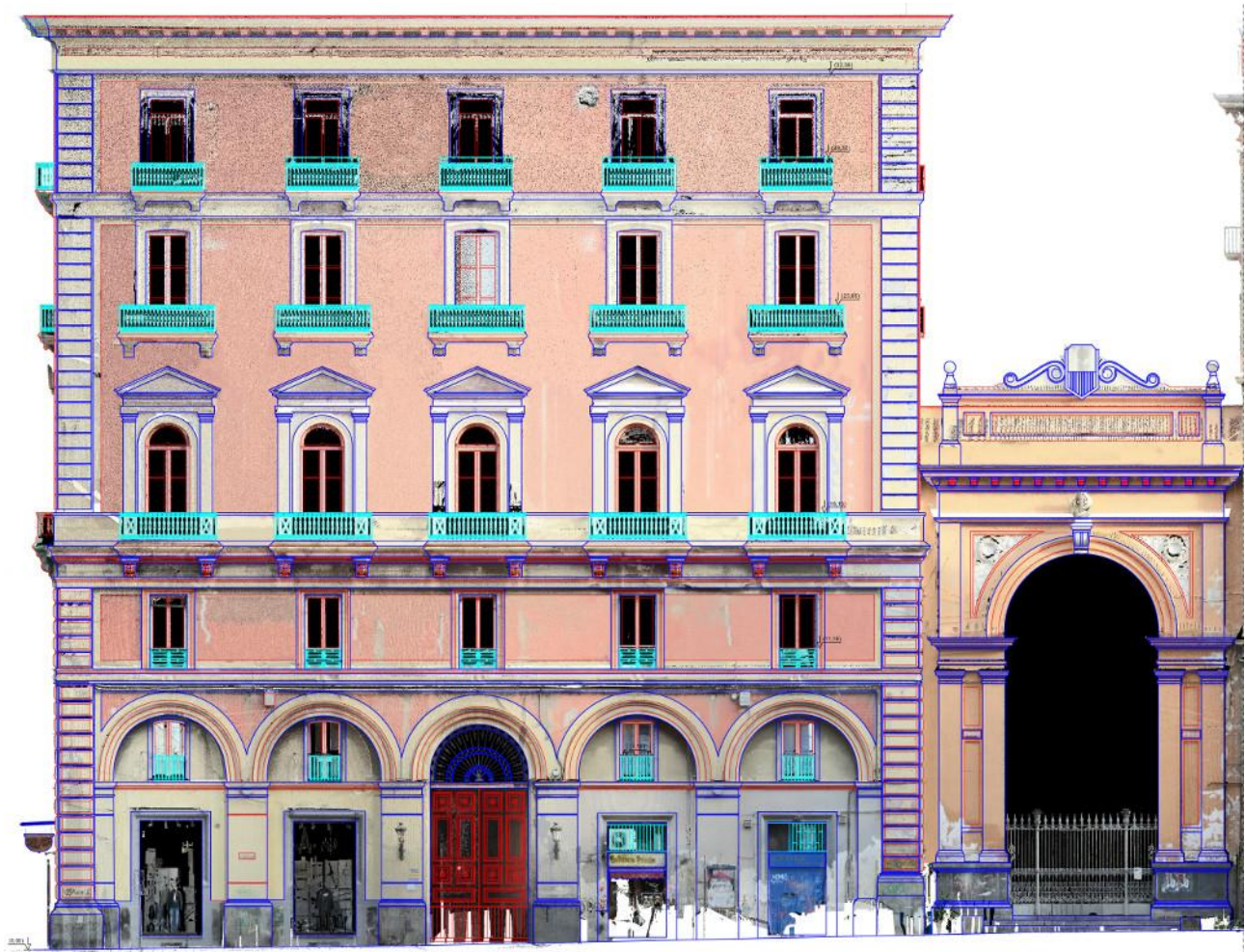
Figure 4: Laser-scanner survey of a 18th century building. Source: Sgobbo, 2015
