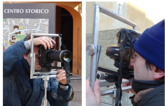
Figure 8. The cardan joint based rotating camera system.
