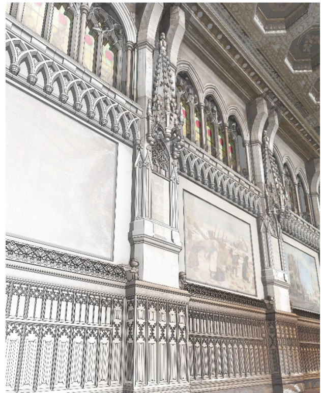
Figure 4. The Senate Chamber BIM at LOD 4
