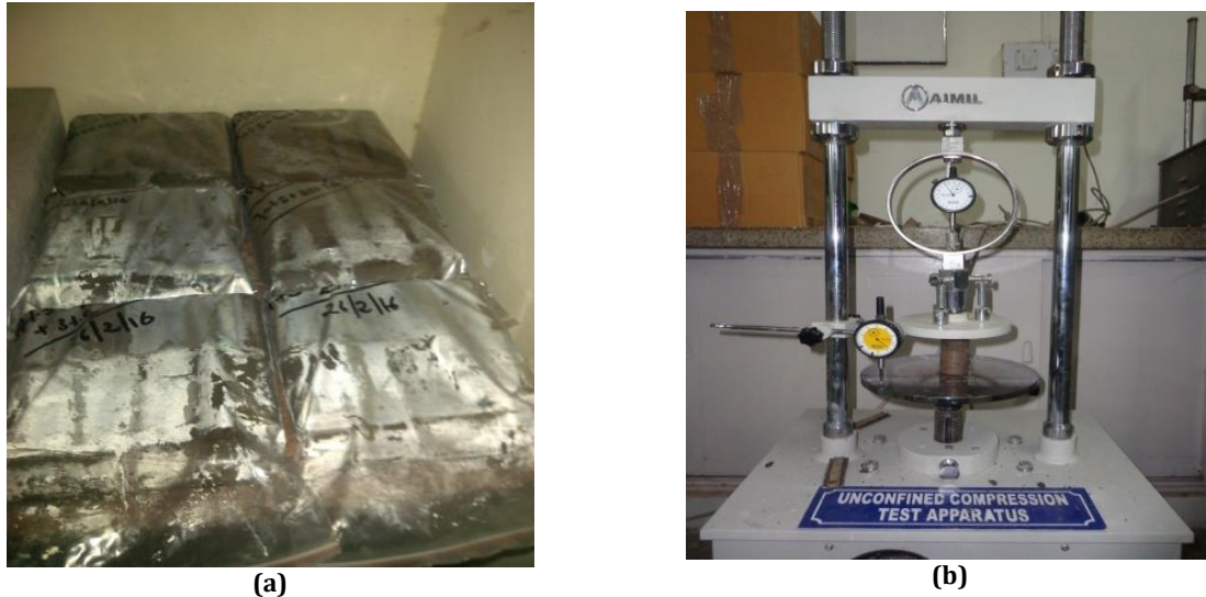
Fig 3. (a) Specimens cured in humidity-controlled room (b) Setup for unconfined compressive strength tests
