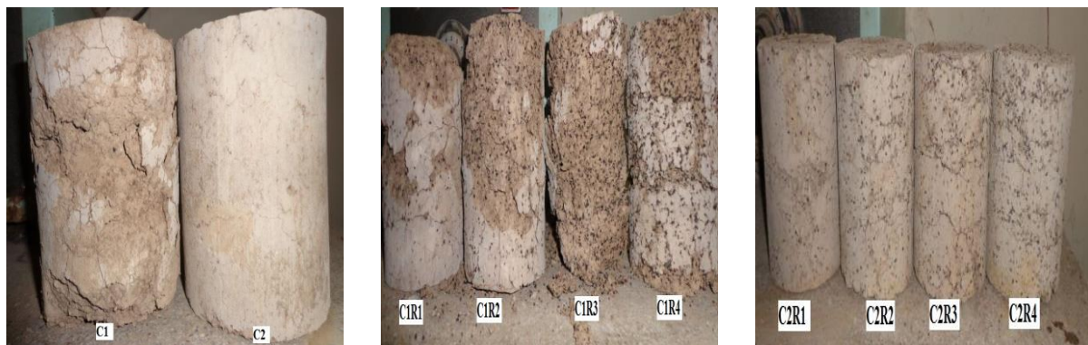
Fig 11. Photographs of the composite cured for 180 days during wetting and drying cycles.
