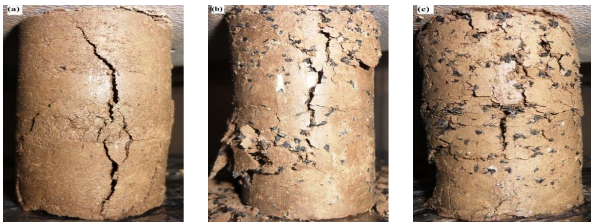
Fig 8. (a) Vertical cracking in cemented clay specimen, (b) & (c) Multiple/staggered cracking in cemented clay specimen containing rubber.
