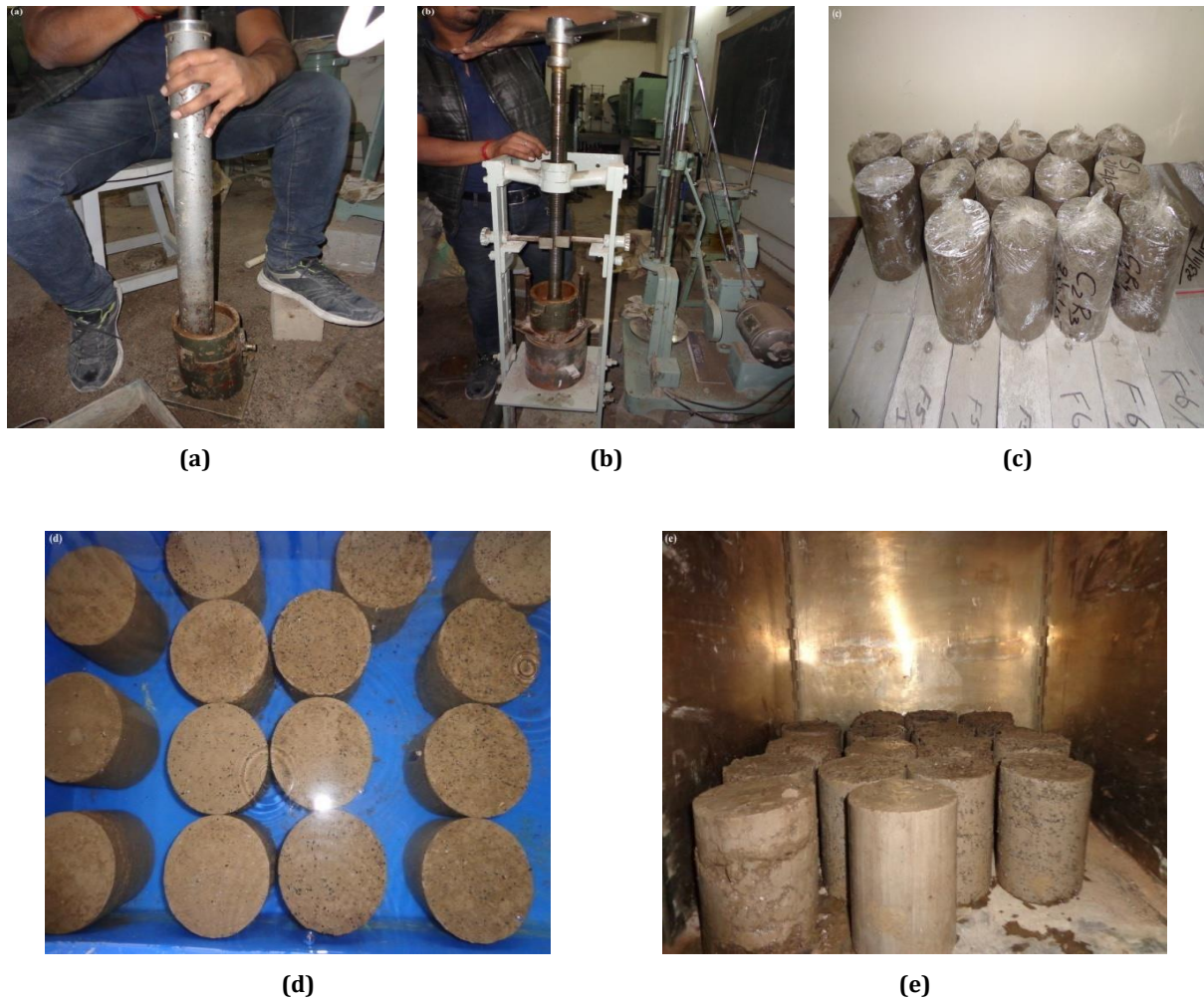
Fig 4. The sequential steps of the preparation of samples for wetting and drying durability testing from: (a) to (e).
