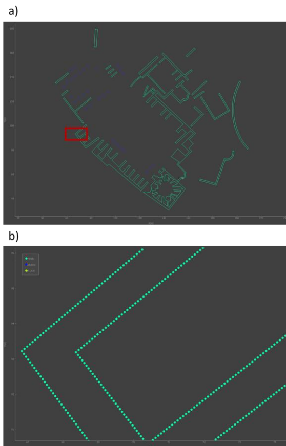
Figure 11. a) 'Herdonia' case study after delineation and discretization, b) a visualization of a small area to observe the discretization.
