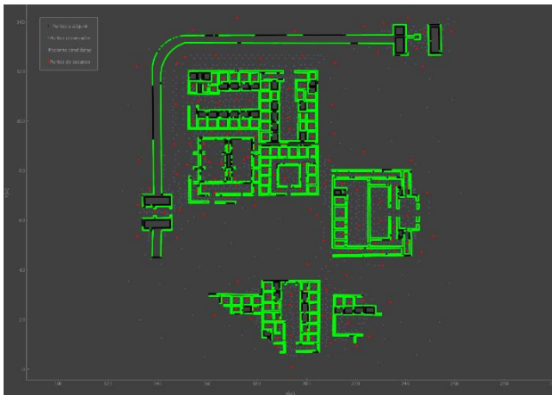
Figure 7. Candidate positions (in grey), scanning positions (in red) and scanned points (in green).
