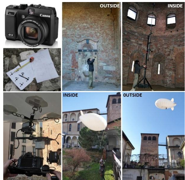
Figure 4 Aerial and terrestrial photogrammetry
