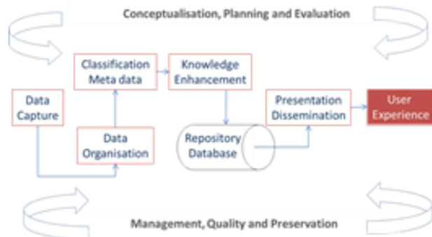
Figure 9: System Architecture for Archival and Storage Repository
