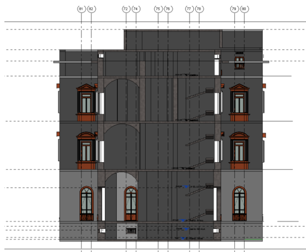
Figure 10 Naples Section of the Federico II building on the main staircase. 3D model (2018)
