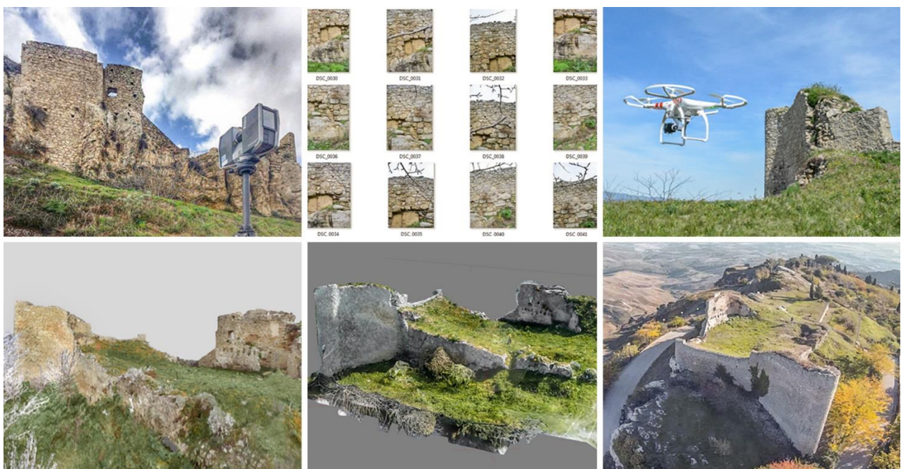
Figure 3. The integrated survey: 3D laser scanning and digital terrestrial and UAV photogrammetry
