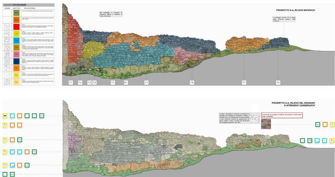
Figure 5. The wall masonry characterisation, the decay mapping and the conservation project
