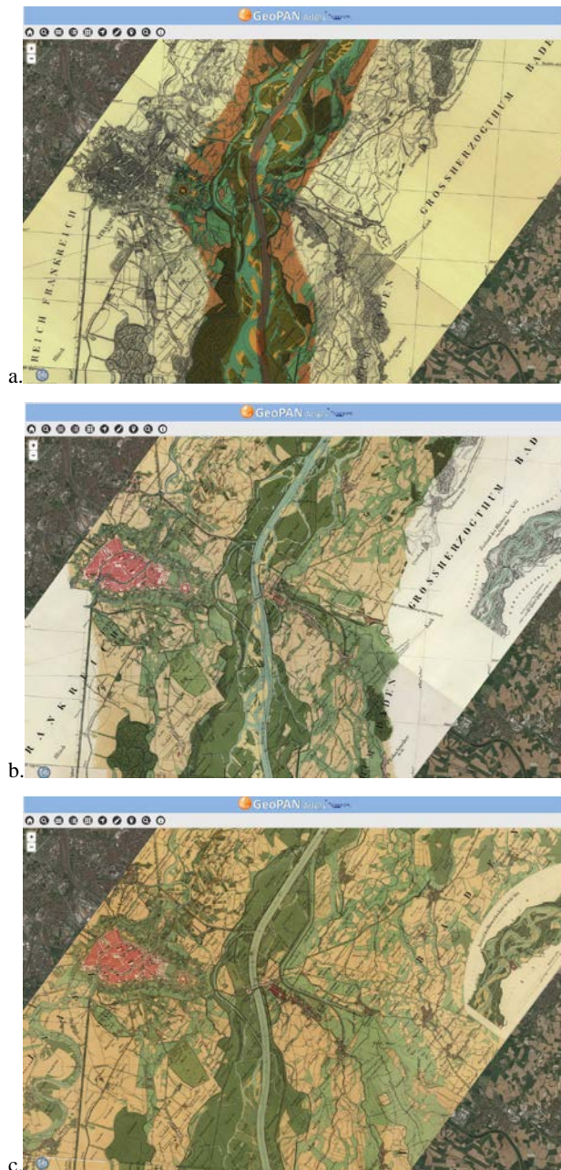
Figure 5. Rhine river in correspondence of Strasbourg: the original riverbed in 1830 (light blue) and the rectification project (red) (a), the riverbed (light blue) in 1852 (b) and 1872 (c).
