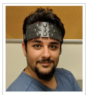
**FIGURE 2** | fNIR<sup>®</sup> sensor pad used for data collection. Written informed consent was obtained from the individual to publish this image.
