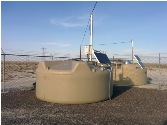
Figure 2. Two Auger Water Cherenkov Detector (WCD) surface detector stations deployed at the Central Laser Facility (CLF) of the Telescope Array (TA) corresponding to Phase I for Auger@TA: Auger North (near) and Auger South (far).
