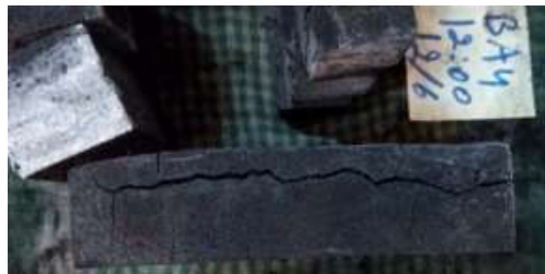
Fig. 4. Crack Development due to Curing for High Content of Fly Ash
