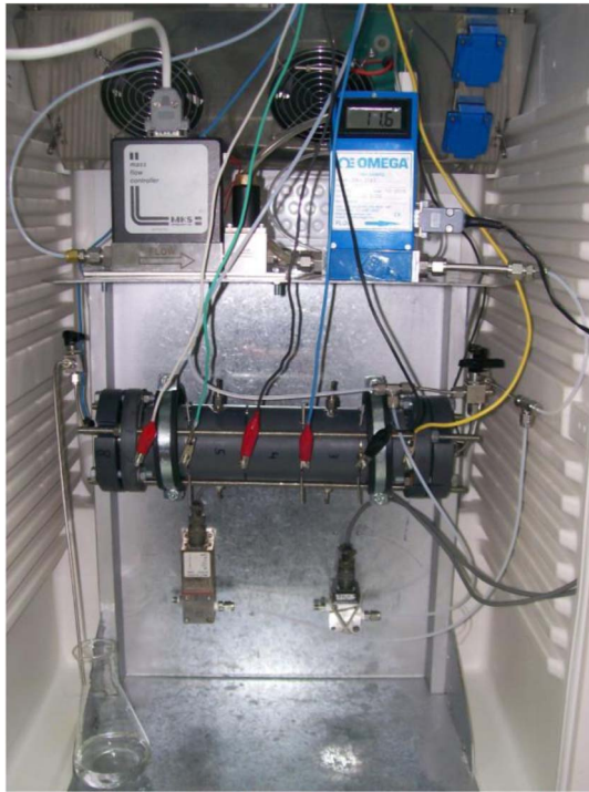
Fig. 2. Sand column equipped with two pressure transducers, a gas mass flow controller, and six electrodes.
