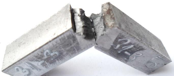
Fig. 8. Sample with V-notch at welded joint after testing of impact toughness
