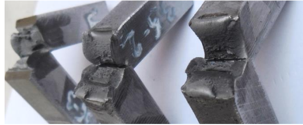
Fig. 15. Appearance of fracture surface after testing of samples notched in HAZ
