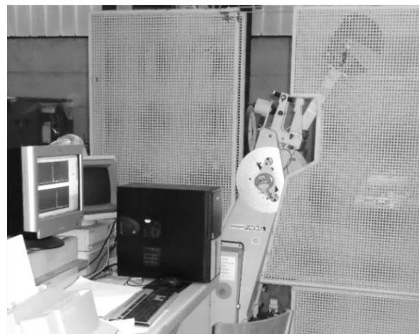
Fig. 5. Computerized Charpy pendulum used for testing
