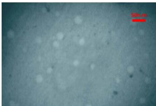
Figure 1. TEM image of nanomicelles. Diluted nanomicelles (20 \mu l) were deposited onto carbon coated copper grid. After 1 minute, the excess nanomicelles was removed by filter paper (Whatman®) and stained with 10 \mu l of 1 % sodium phosphotungstate pH 7.0 for 2 min. The samples were photographed with a Phillips CM100 electron microscope (Philips/FEI Corporation, Eindhoven, Holland)
