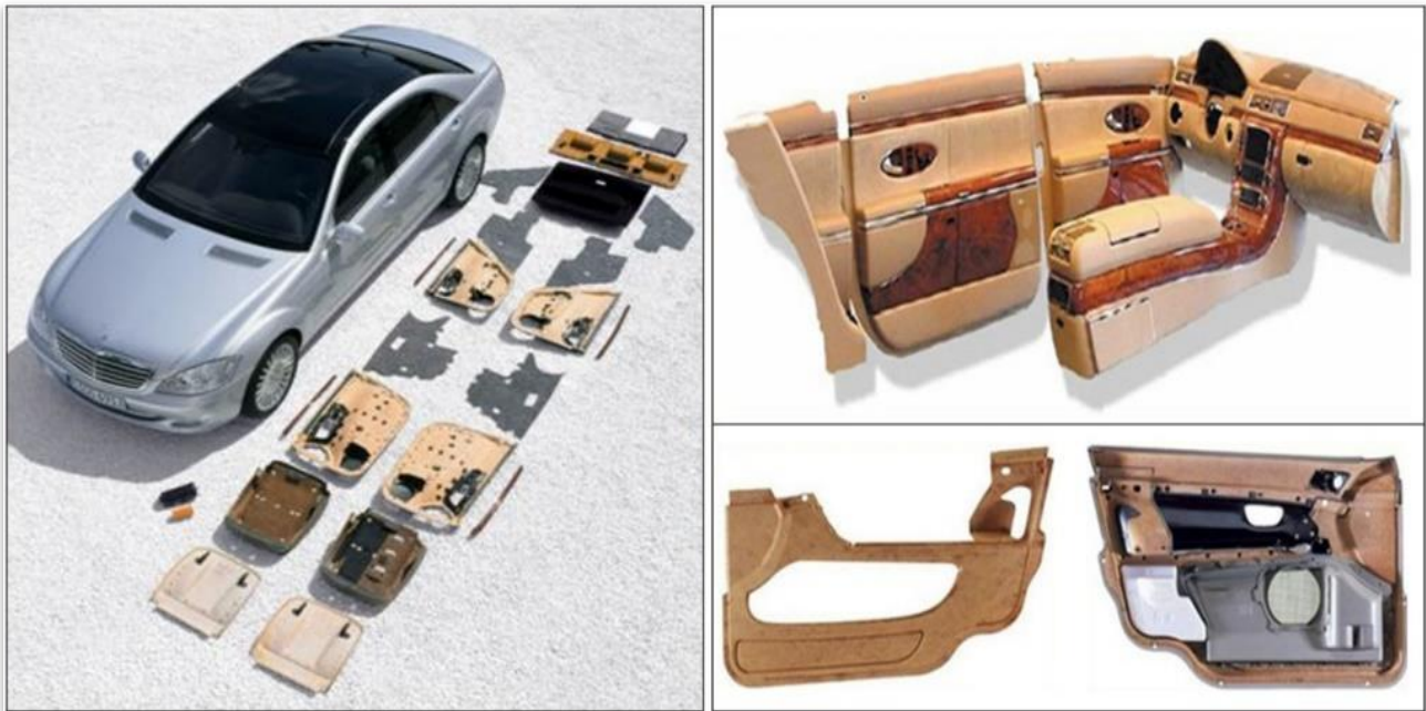
Fig. 4. The use of natural fibers for technical composite applications in automotive industries
