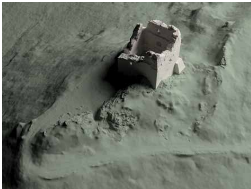
Fig. 10. Přimda. A 3D model of the Romanesque keep based on the LLS and ground scanning. Based on Sokol, 2015, p. 70.
