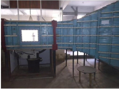
Fig. 2b. Open type sub-sonic wind tunnel.
