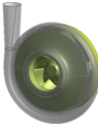
Fig. 2. Assembly view of the centrifugal pump.
