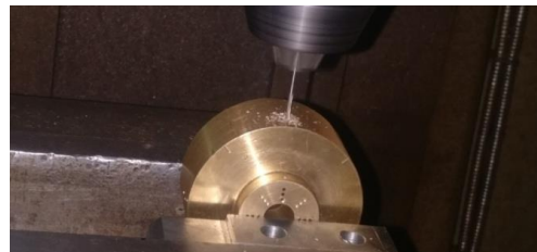
Fig. 5. Drilling holes for control jets on a radial drilling machine.
